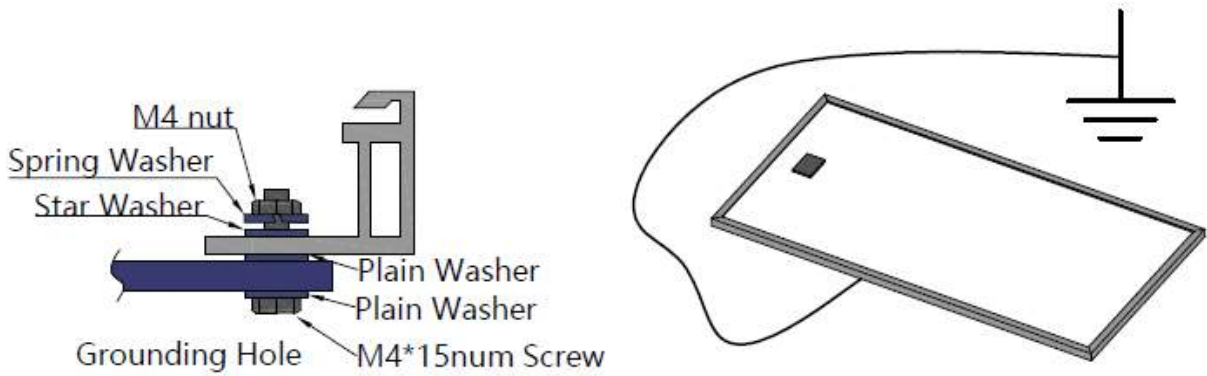
Figure 10: Ground installation of PV modules
